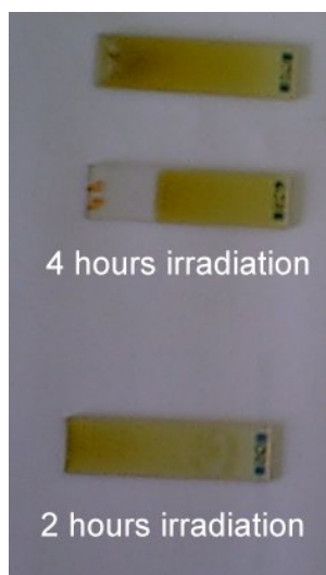
Figure 1 : view of different films of tholins used for optical characterization. These samples have been obtained by depositing organic aerosol particles on a quartz plate inserted in a plasma flow, where the particles are in situ synthesised.
